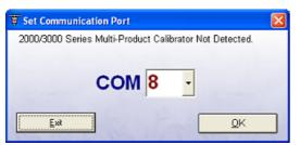
If the 3000 Series VFP is not detected, or no COM port has been chosen before, the COM select screen will be displayed.
